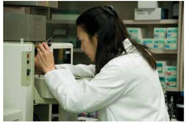
Laboratory Analyst sets up the Atomic Absorption Spectrophotometer.
